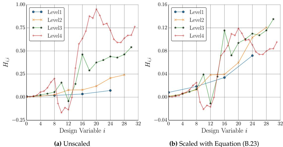
**Figure B.3: 3D off-body pressure functional:** Hessian diagonal at various shape control resolutions. Left to right traverses the radius control stations from tip of forebody to the base (see Figure 5.18).
