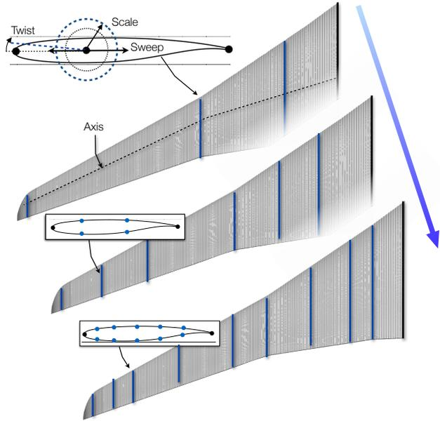
**Figure 1.1:** Notional parameterization refinement for wing design.
