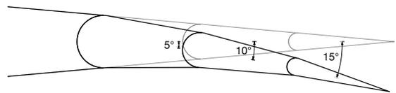
(b) Each flap can be segmented, allowing more precise re-cambering.
