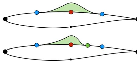
**Figure 3.1:** Under an interpolation-based deformation model, the red parameter’s deformation mode shape (and thus the potential it offers) depends on the location of its neighbors.
