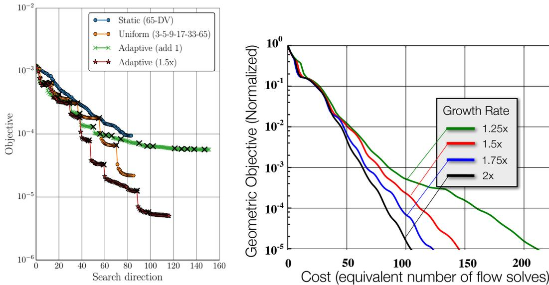
(a) Supersonic inverse design to off-body target pressure signature.  $\times$ -marks denote search space refinements. (b) Geometric shape-matching objective. Each curve shows mean behavior of 10 randomized trials ( $r = 0.25$ ).
