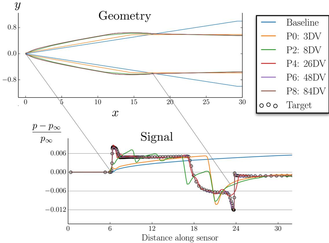
(a) Signature recovery throughout adaptive parameterization (for clarity, not all intermediate signals are displayed)
