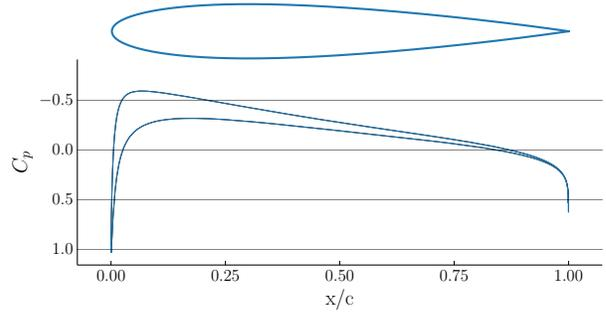
**Figure 5.8: Inverse Airfoil Design:** Target airfoil (NACA 0012) and pressure profile.  $Mach\ 0.3$ ,  $\alpha = 1^\circ$
