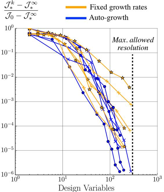
**Figure 5.13: Inverse Airfoil Design:** Convergence to continuous optimum using both fixed growth rates (orange) and automatically determined growth rates (blue). Objective values are normalized to begin at  $\mathcal{J}_0 = 1$ , to remove the discrepancy in  $\mathcal{J}_0$  for the different starting points.
