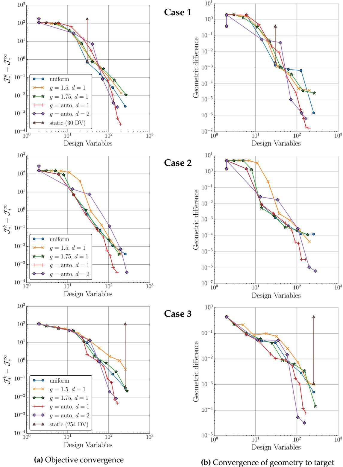
**Figure 5.12: Inverse Airfoil Design:** Convergence of the objective with respect to shape control refinement. Each curve indicates a different refinement strategy. Each point indicates the best (final) objective value attained within that level.
