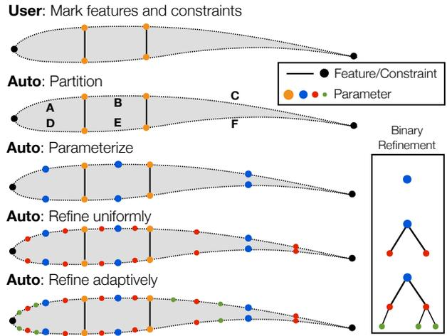
**Figure 2.5:** Progressive parameterization with discrete, hierarchical shape control refinement
