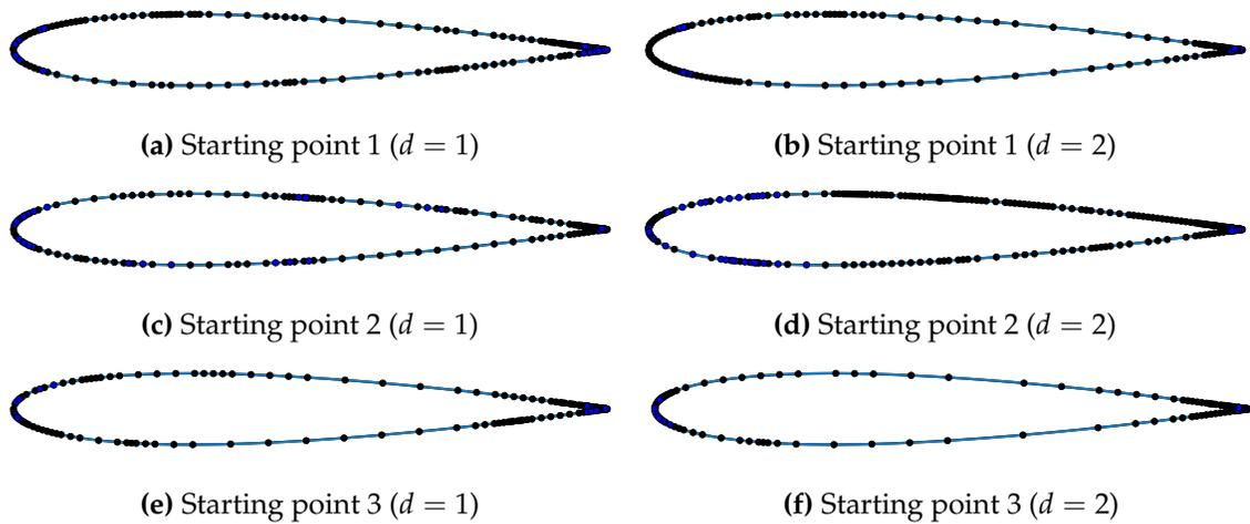
**Figure 5.15: Inverse Airfoil Design:** Final adapted parameterizations for each starting point, using two auto-growth strategies.
