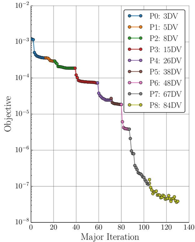
**Figure 5.20:** *Supersonic Forebody*: Objective convergence (adaptive parameterization strategy)
