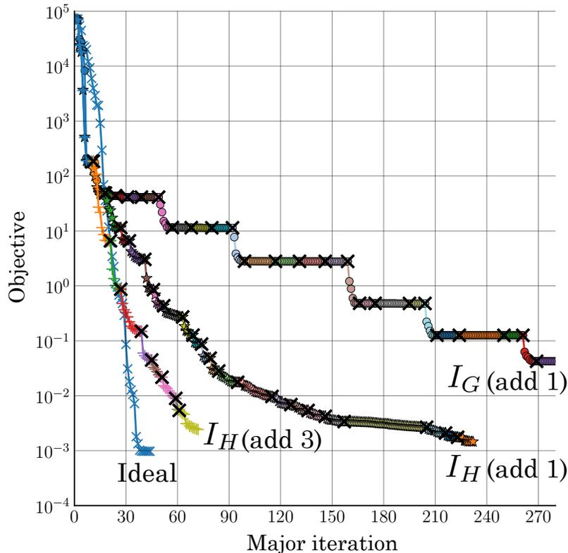
**Figure 5.6: Shape Matching:** Objective convergence with different indicators and adaptation strategies. Each color represents a suboptimization, and  $\times$ -marks denote search space refinements. The curve labeled “Ideal” represents the most efficient possible 35-DV parameterization.
