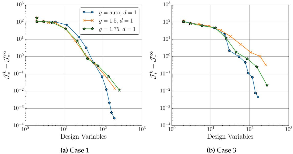
**Figure 3.8:** Performance of automatic growth vs. fixed growth rate on 2D inverse design example (more details in Section 5.2). Each curve indicates a different refinement strategy. Each datapoint indicates the best objective value attained within a suboptimization level of Algorithm A.
