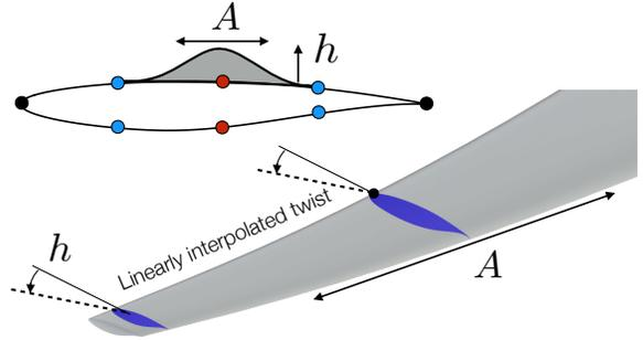
**Figure 3.3:** Shape mode characteristic dimensions  $A$  and  $h$  for two parameterization techniques. For the twist case,  $h$  might indicate, e.g.  $1^\circ$  twist.
