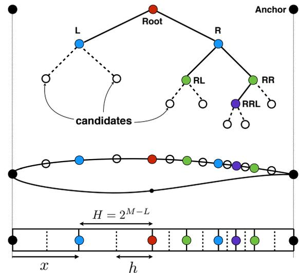
**Figure 2.7:** Binary tree and grid representations of an airfoil shape parameterization, showing candidate refinement locations computed by Function 3 in Appendix A
