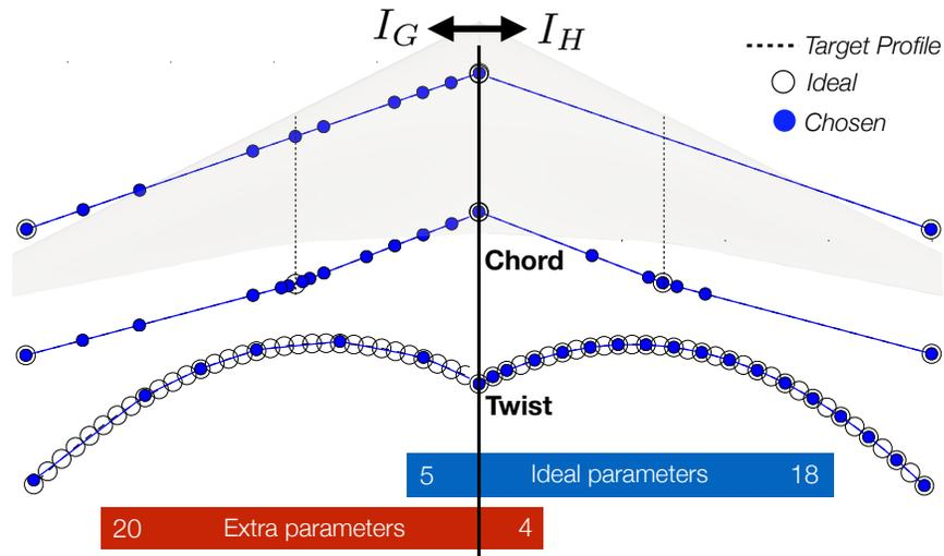
**Figure 5.5: Shape Matching: Test 1:** Final adapted parameterizations using  $I_G$  (left) vs.  $I_H$  (right).  $I_H$  recovers the expected parameters with few extras, while  $I_G$  mostly adds extraneous parameters.
