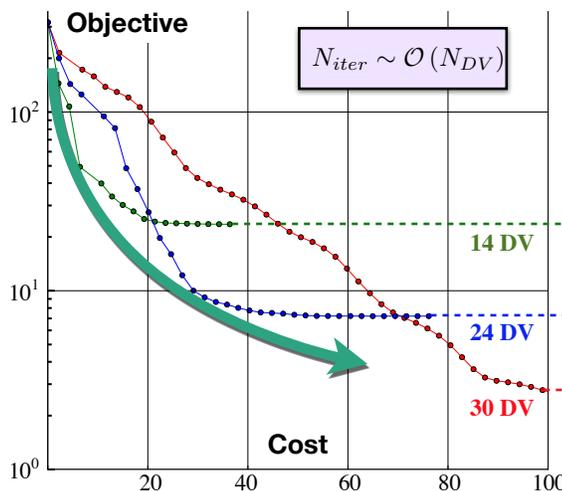
**Figure 2.2:** Static parameterizations compromise between efficiency and performance of the optimal design. A progressive parameterization approach dynamically controls  $N_{DV}$ , allowing the process make rapid gains early, while approaching the continuous optimal shape. The goal is to follow the “inside track”, notionally illustrated by the green arrow. Data corresponds to a geometric shape matching optimization.
