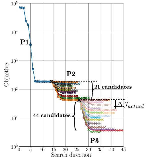
**Figure 5.2: Shape Matching: Indicator verification:** **P1:** Objective convergence under initial parameterization. **P2** and **P3:** Subsequent optimizations corresponding to addition of one of the candidates, starting from the previous best design.
