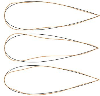
**Figure 5.11: Inverse Airfoil Design: Robustness Study:** Randomly-generated initial geometries (1-3 from top to bottom)
