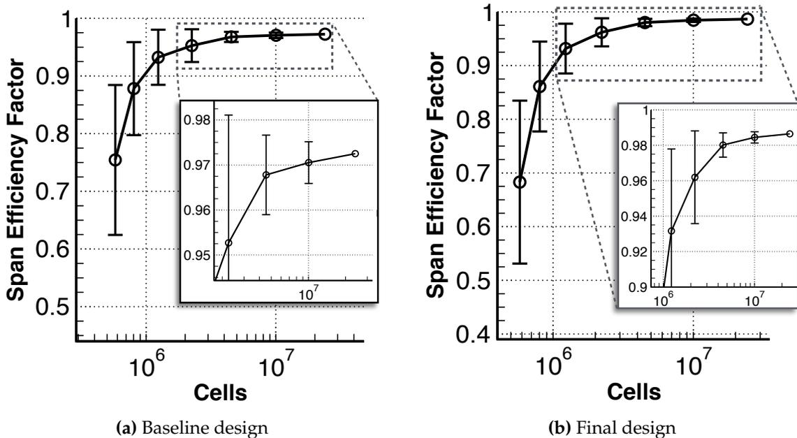
Figure 6.6: *Twist optimization*: Convergence of span efficiency factor with mesh refinement
