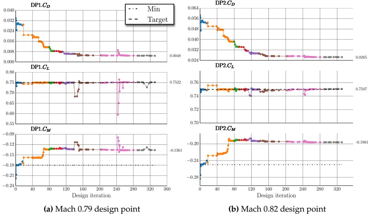
**Figure 6.11: Transonic Airfoil:** Convergence of aerodynamic functionals across all adaptively refined parameterization levels (2-DV in blue, 4-DV in orange, etc.). Target/minimum constraint values shown in dashed lines.
