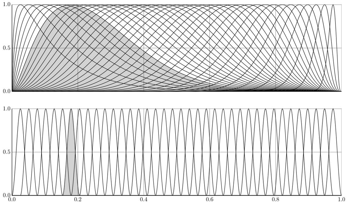
**Figure 4.2:** Local vs. global mode shapes. Plotted are shape modes for 18 evenly-spaced centers. One corresponding pair of modes is highlighted. *Top:* Hicks-Henne bump functions ( $y = \sin^4(\pi x^{\frac{\log 0.5}{\log x_j}})$ ). *Bottom:* Local cubic blending functions ( $y = 2|x - x_j|^3 - 3|x - x_j|^2 + 1$ ).
