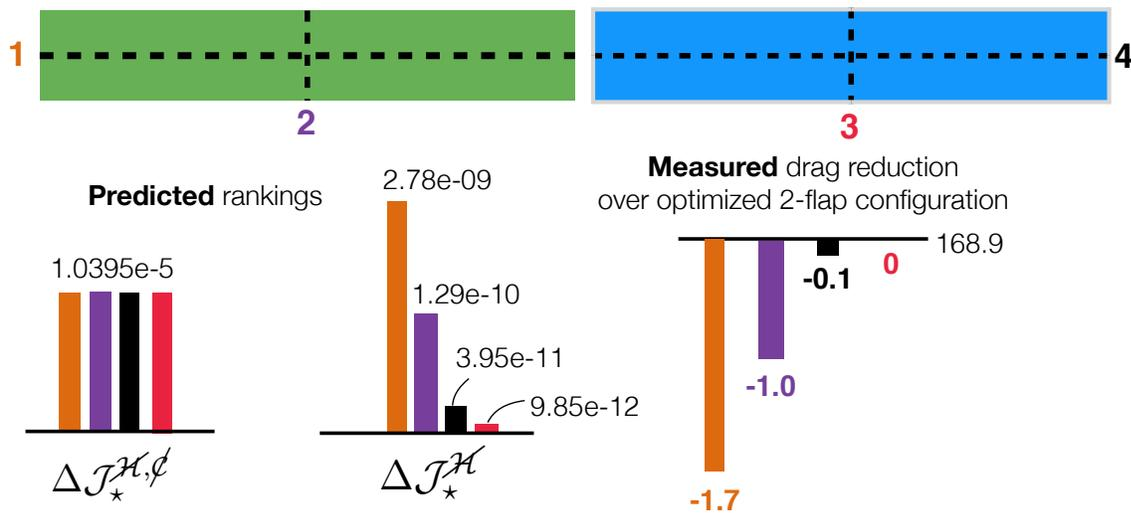
**Figure 6.15: Truss-braced Wing:** The adaptive system ranks the four initial candidate flap subdivisions using  $I_G$ , both accounting for and neglecting constraints. The version accounting for  $C_L$  provides a correct relative ranking of the candidates, as demonstrated by the actual drag recovery obtained by optimization. (Drag values are in counts, trimmed to  $C_L$  constraint.)
