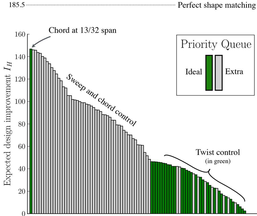
**Figure 5.7: Shape Matching: Test 3:** Initial priority queue ( $d = 5$ ,  $N_{add} = 32$ ,  $I_H$ ). The 32 parameters that would best recover the target shape (*green*) are highlighted. After adding the top member of the queue, all of the subsequent chord and sweep controllers (*gray*) become redundant.
