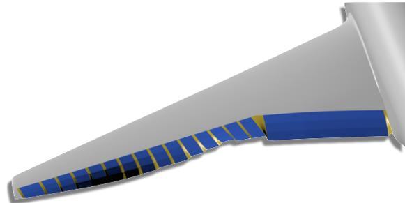
(a) One possible flap system built using the modeler. Blue regions are flaps, gold are joining elastomer material.
