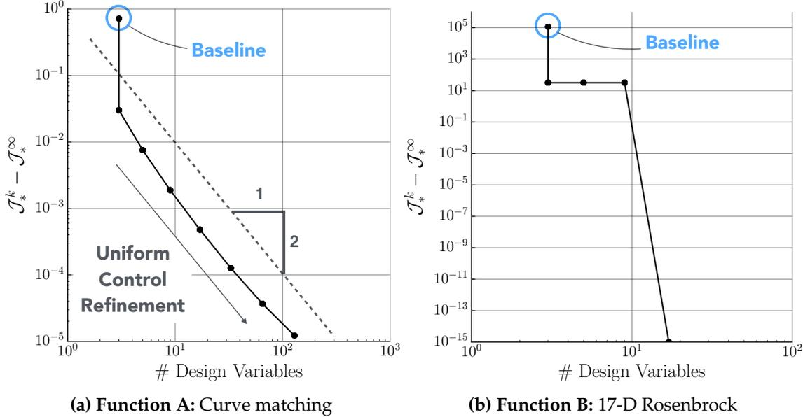
**Figure 2.3:** Convergence to the continuous optimum with refinement of the control variables. Each data point represents a full optimization in a discretized search space.
