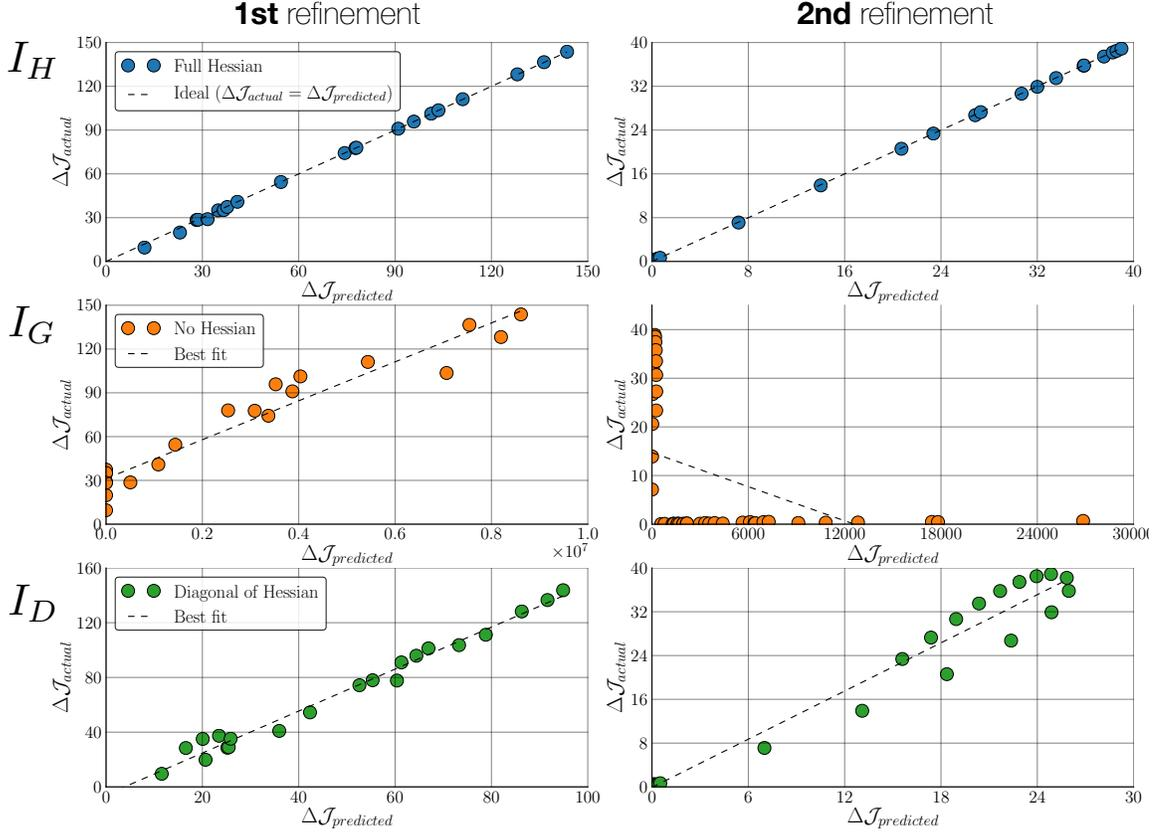
**Figure 5.3: Shape Matching: Indicator verification:** Correlation between predicted and actual design improvement for the first (*left*) and second (*right*) refinements. *Top row:  $I_H$ , Middle row:  $I_G$ , Bottom row:  $I_D$*
