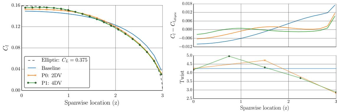
(a) Left: Sectional lift distribution profiles. Top right: Deviation from elliptic distribution. Bottom right: Twist distribution (twist is in degrees and indicates local angle of attack ( $\alpha_{global} + \gamma$ ))
