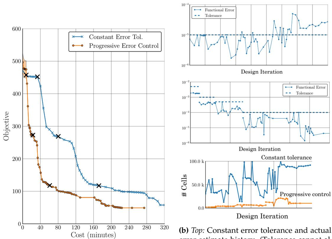
(a) Design improvement vs. wall-clock time (excluding geometry generation). Shaded bands indicate uncertainty due to discretization error.  $\times$ -marks denote search space refinements.
