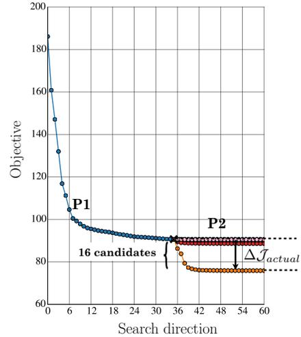
**Figure 5.9: Inverse Airfoil Design: Indicator verification:** Objective convergence under initial parameterization, followed by subsequent optimizations corresponding to addition of one of the candidates.
