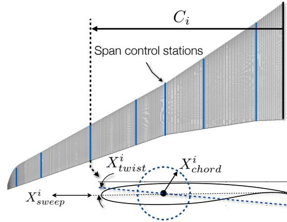
Figure 2.1: Wing planform parameterization
