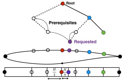
**Figure 3.9:** Regularity prerequisites for airfoil parameterization. Addition of the requested parameter (in purple) would lead to excessive variation in parameter spacing. The system automatically adds its two prerequisites. One of those, in turn, requires addition of a third parameter.
