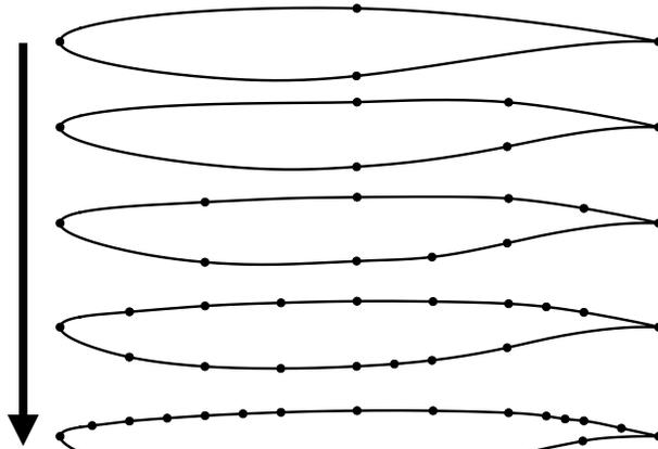
**Figure 6.10:** *Transonic Airfoil:* History of adaptive refinement, showing best airfoils attained under the first several parameterizations.
