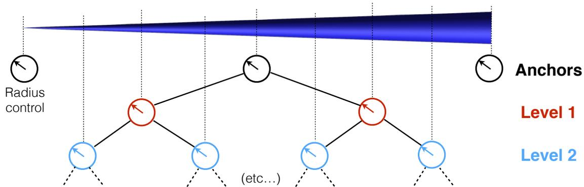
Figure 5.18: *Supersonic Forebody*: Hierarchical shape parameterization of forebody radius
