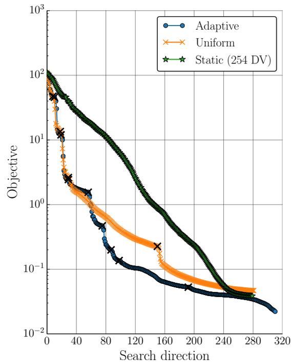
**Figure 5.14: Inverse Airfoil Design:** Objective convergence with respect to design iteration. When given an aggressive trigger, progressive schemes tend to exhibit faster convergence than a static parameterization. Adaptive refinement substantially outperforms uniform refinement.
