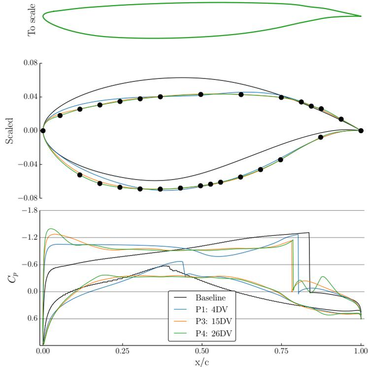
**Figure 6.9: Transonic Airfoil:** Optimization results for the adaptive parameterization approach. *Top:* Optimized airfoil to scale. *Middle:* Final airfoil from three intermediate search spaces (4-DV, 15-DV, 26-DV), showing 26-DV adapted parameterization. *Bottom:* Corresponding pressure profiles for the Mach 0.79 design point.
