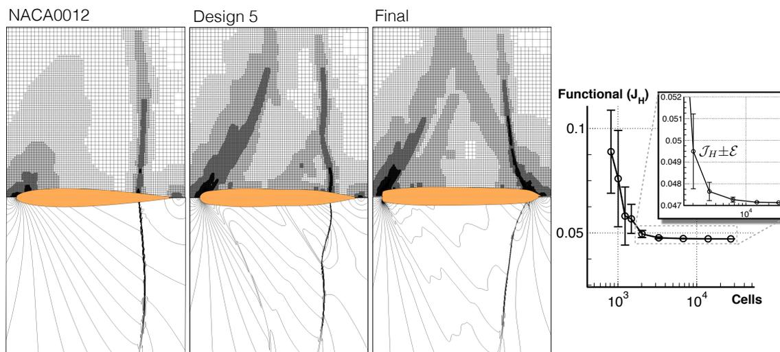
**Figure C.1: Symmetric Airfoil:** (See Section 6.1 for case details.) *Top:* Flow meshes adapted to accurately compute pressure drag for three airfoils encountered during optimization. *Bottom:* Mach contours. *Right:* Convergence of drag functional with mesh refinement for the baseline. Bars indicate uncertainty in drag and asymptotically bound the actual changes in the functional.
