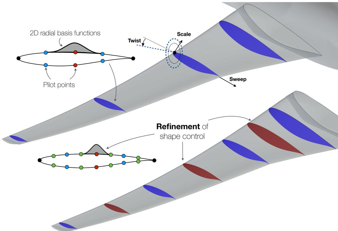
Figure 4.4: Wing deformation model
