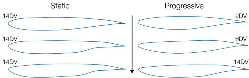
**Figure 6.13: Transonic Airfoil:** Shapes encountered during optimization under a progressive parameterization (*right*) are consistently much smoother than airfoils encountered under a static parameterization (*left*).
