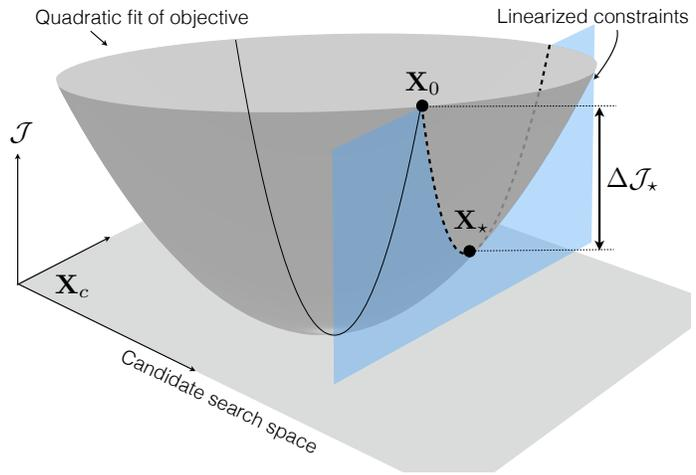
**Figure 3.2:** Estimating feasible design improvement in a candidate search space using a local quadratic fit of the objective and local linearization of the active constraints.
