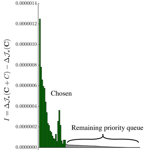
**Figure 3.7:** Reduction of indicator with addition of shape control. The refinement procedure has been terminated after consecutive new shape controllers (green) demonstrated consistently diminished priorities ( $r = 0.1, w = 3$ ).
