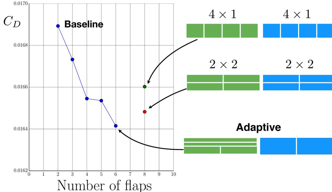
**Figure 6.17: Truss-braced Wing:** Inviscid drag on full configuration, on coarse 12-million cell optimization mesh. Adaptive refinement has uncovered a flap topology that outperforms two reasonable layouts, while using fewer components. In the process it has begun to reveal an approximate tradeoff between drag reduction and number of parts.
