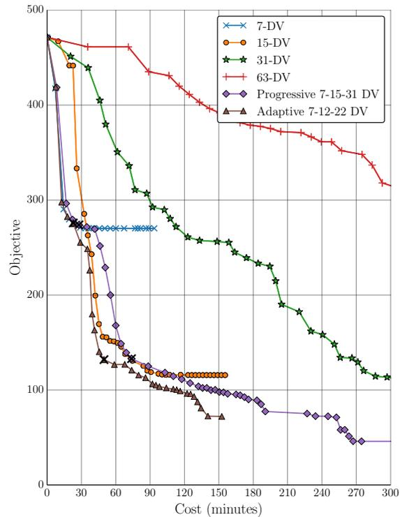
**Figure 6.4:** *Symmetric Airfoil*: Cost-effectiveness of each parameterization scheme, showing design improvement vs. wall-clock time (using late 2013 MacBook Pro, 4 × 2.6GHz Intel Core i7, 16GB of memory). ×-marks indicate search space refinements on the progressive and adaptive methods. All cases used identical settings for meshing, solving, error control and triggering.
