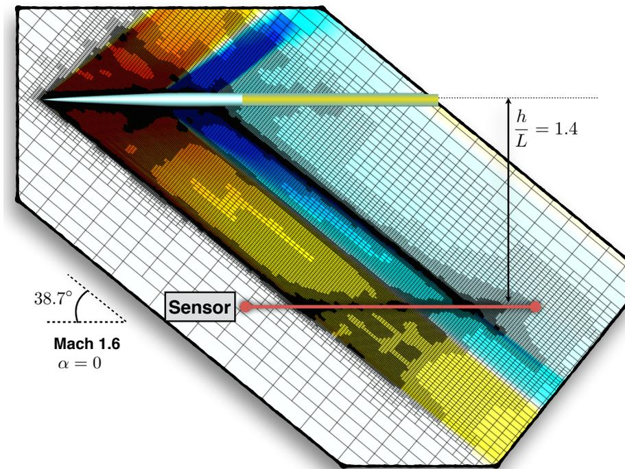
**Figure 5.17: Supersonic Forebody:** Example of an adapted flow mesh. Cells are distributed to accurately compute the pressure signature along the sensor (*orange line*). The mesh shown is for the target shape and has 1.9M cells.
