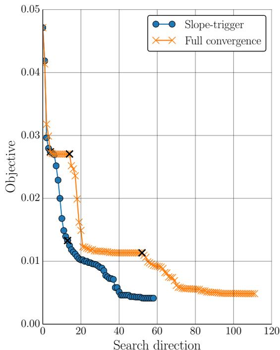
**Figure 2.9:** Orange: Optimizing to convergence on each level leads to slow design improvement. Blue: Using aggressive slope-based transitions permits much faster design improvement.  $\times$ -marks denote parameterization refinements.
