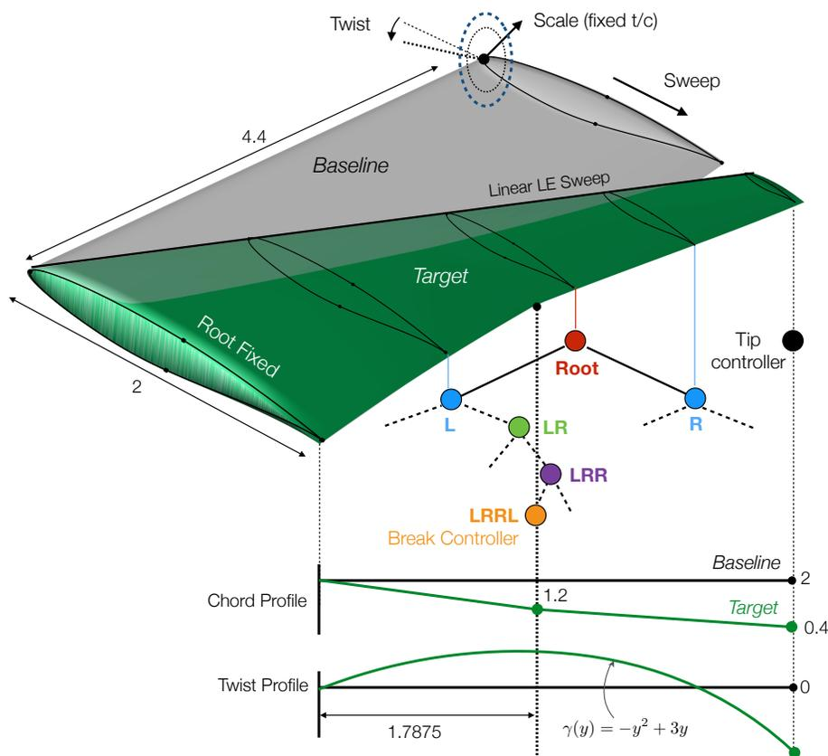
**Figure 5.1: Shape Matching:** Baseline and target planform profiles. Shape control is organized in spanwise tree structure. At a depth of  $d = 4$ , a controller can be added at the wing break.
