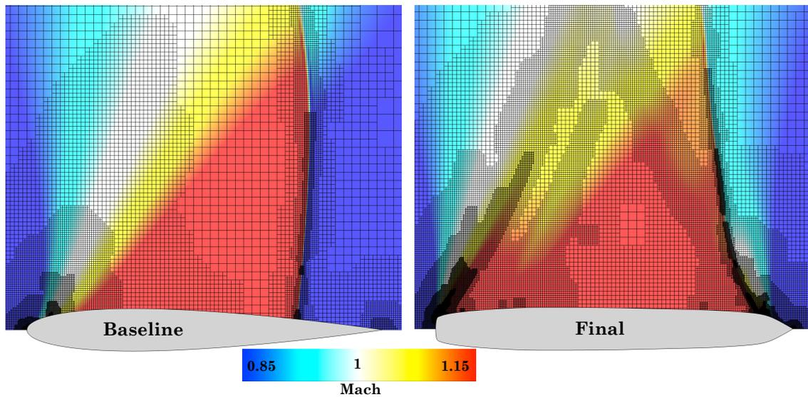
**Figure 6.3: Symmetric Airfoil:** Comparison of baseline and final meshes. The mesh refines the regions most important for computing drag, primarily focusing on the leading edge expansion and shock. To achieve the same error tolerance for both designs, the baseline mesh required only 26K cells (upper half only), while the final design required 61K cells.
