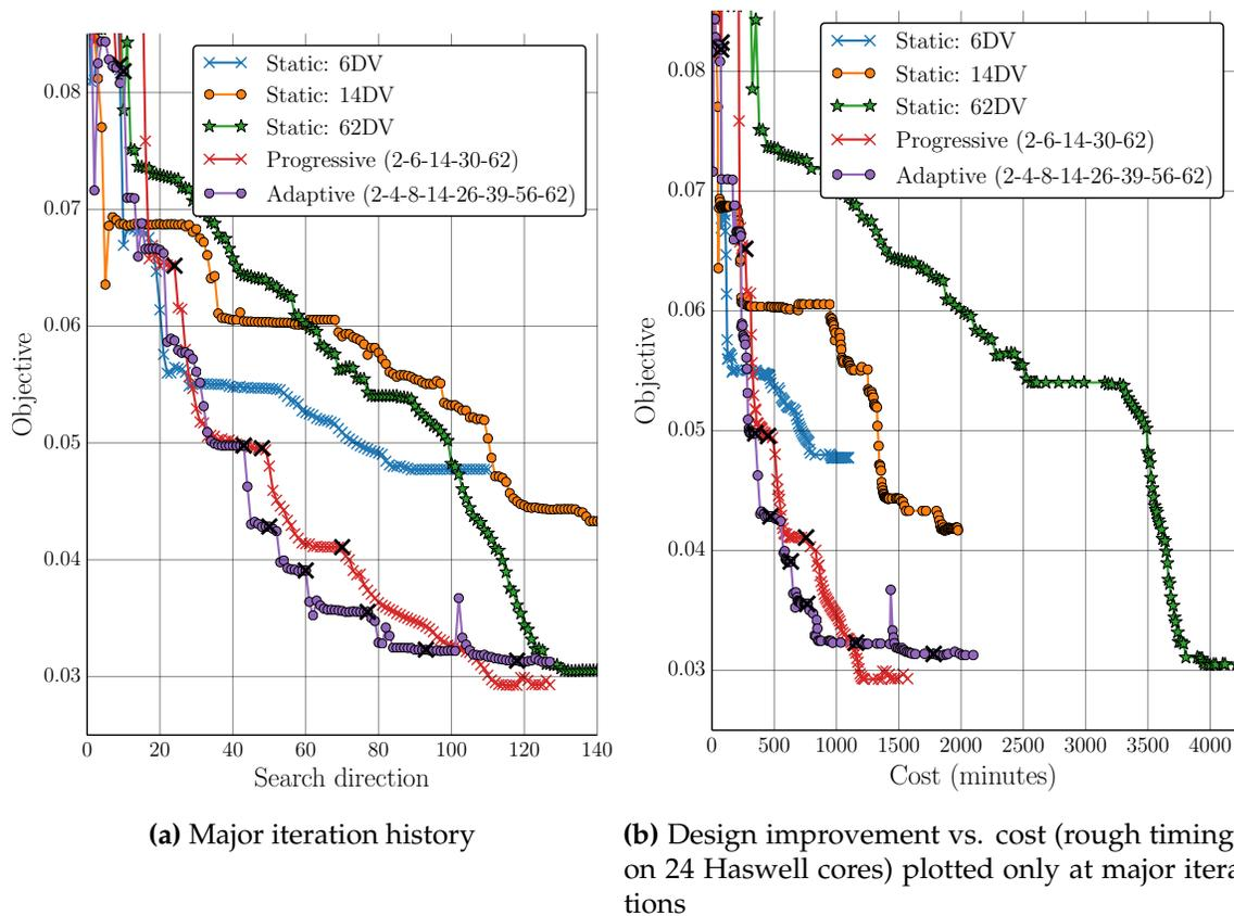
**Figure 6.12: Transonic Airfoil:** Convergence of combined drag value ( $C_{D_1} + C_{D_2}$ ) (ignoring satisfaction of constraints) for each parameterization method.  $\times$ -marks denote search space refinements.
