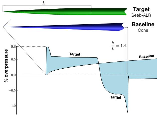
**Figure 5.16: Supersonic Forebody:** Baseline and target geometries and corresponding off-body pressure signatures (*off-body distance not to scale*). Shaded region indicates the signal deviation to be driven to zero by shape optimization.
