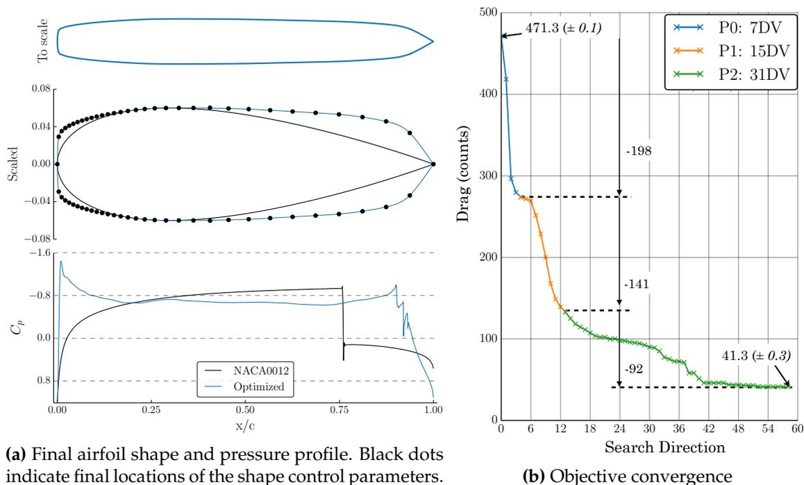
Figure 6.2: *Symmetric Airfoil*: Progressive parameterization optimization results
