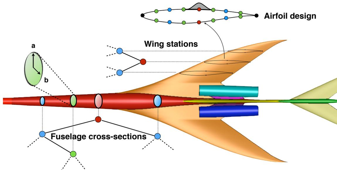
Figure 2.6: Progressive parameterization of an aircraft configuration
