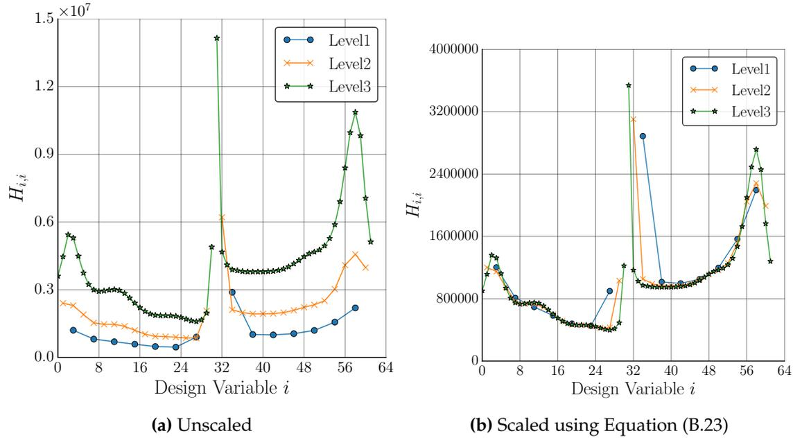
**Figure 3.4:** Hessian diagonal for 2D inverse pressure matching on airfoil at various shape control resolutions. Left/right segments on each plot correspond to camber/thickness. Trailing edge is at the center, leading edge on either side.
