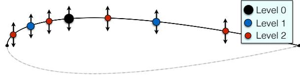
**Figure 6.1: Symmetric Airfoil:** Initial parameterization with 7 design variables, generated by twice uniformly refining a 1-DV parameterization (lower half generated by symmetry)
